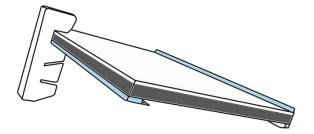
2. Place the cheiroscope tiltfoot on the left rear of the tiltboard kit.
