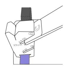
6. Insert magnet onto the foam end of mirror with the magnet facing up.
