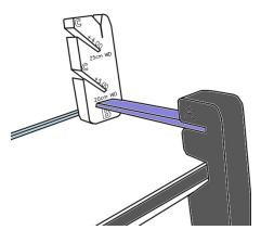
5. Insert the "C" end of the mirror, with the mirror side facing up, into either the +4.00 or +5.00 "C" slots of the mirror mount according to your activity's needs.
