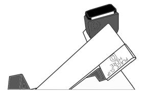
7. Insert the charts into the vertical slot at the top of part mirror mount. \*Note: charts stay more rigid if you place 2-4 charts in the slot at a time.
