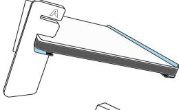
3. Insert the foam side "A" of the blue stick firmly into the "A" slot in the cheiroscope tiltfoot.
