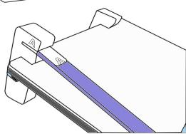
4. Orient the mirror mount vertically with the lettering oriented upright and the flat side of the mirror mount facing the left. Slide the "B" slot of the mirror mount over the "B" end of the blue stick. Slide the mirror mount to approximately half the length of the blue stick.
