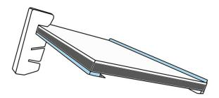
2. Place the cheiroscope tiltfoot on the left rear of the tiltboard kit.
