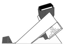
7. Insert the chart into the vertical slot at the top part of the mirror mount (Note: charts stay more rigid if you place 2-4 charts in the slot at a time). Charts are designed for either Right Eye or Left Eye orientation (see introductory note). If the image is upside down then it was designed for the other Eye orientation. However, presenting the image upside down can provide an additional load for patients.
